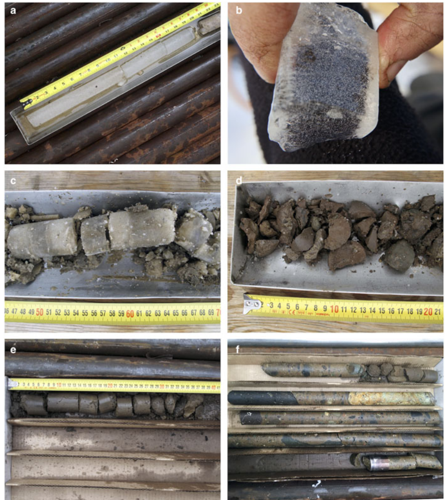
Fig. 10. Photographs of cored materials recovered in hole 2. (a) Dirty glacial ice below 677 m with flecks of rock debris. (b) Close-up of glacial ice containing air bubbles. (c) Dirty, banded ice from ~678 m. (d) Soft, gritty till containing pebbles. (e) Hard, dry, compacted till (surface is wet from drilling fluid). (f) Bedrock core of heterolithic tillite from ~679–681 m. Measuring tape in cm.
