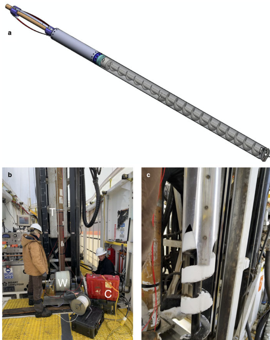
Fig. 7. Chip bailer used to clear cuttings from the auger borehole. (a) CAD model of the IDP 4-in Drill fitted with the chip bailer auger and head. The outer tube of the drill barrel is shown transparent in order to show the chip bailer auger assembly. (b) The IDP 4-in drill winch (W), tower (T) and control box (C) set up on the RAID work deck. (c) Chip bailer, in process of unloading cuttings, consisting of a steel barrel housing internal screw flights.
