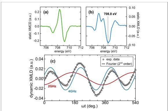
**Figure 3.** Static (a) XMCD and (b) XMLD spectra taken at the Fe  $L_3$  edge of NZAFO. (c) Dynamic XMLD phase delay scan taken with vertically polarized ( $\phi_0 = 0^\circ$ ) x-rays at E = 708.8 eV. The experimental data is fitted with a Fourier extension to 2nd order and evaluated for its 1st (2 GHz, red) and 2nd harmonic (4 GHz, blue) components.
