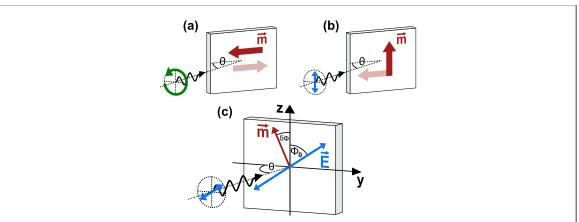
Figure 1. Standard experimental geometry for (a) static XMCD and (b) static XMLD measurements. (c) Schematic of the dynamic XMLD measurement geometry.
