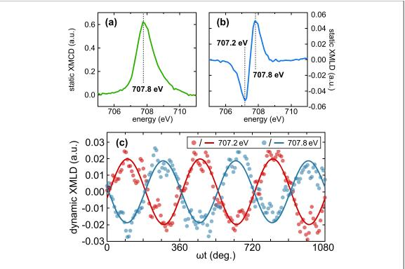
**Figure 2.** Static (a) XMCD and (b) XMLD spectra taken at the Fe  $L_3$  edge of Py. (c) Dynamic XMLD phase delay scans (circles) taken at 707.2 eV and 707.8 eV with 45° x-ray polarization and corresponding sinusoidal fits (lines).
