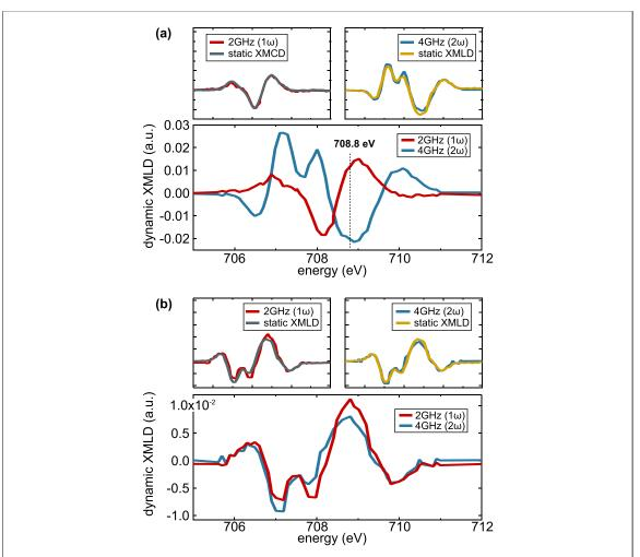
**Figure 4.** Dynamic signal as a function of energy taken at the Fe  $L_3$  edge of NZAFO with (a) vertically ( $\phi_0 = 0^\circ$ ) and (b) horizontally ( $\phi_0 = 90^\circ$ ) polarized x-rays. For vertical polarization the 4 GHz component corresponds to the contribution from dynamic XMLD while the 2 GHz components can be attributed to a spurious dynamic XMCD signal. For horizontal x-ray polarization, both components show a pronounced XMLD lineshape.
