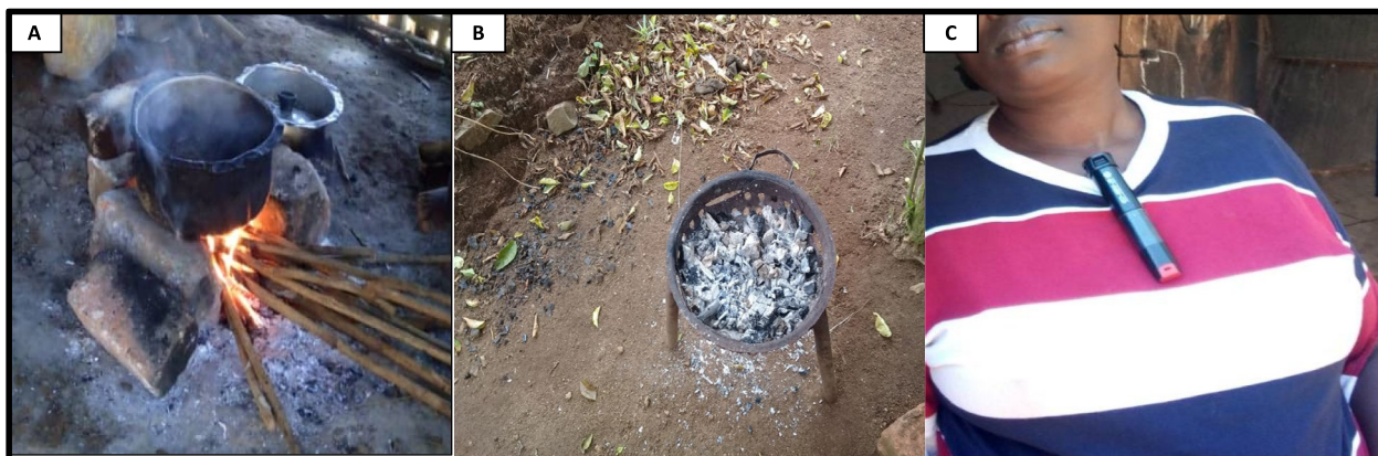
Fig. 2 Panel A traditional “three stones” cooking using wood. Panel B “mbambula” cookstove using charcoal. Panel C woman wearing a Lascar CO monitor
