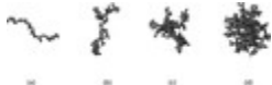
FIG. 1. Conceptual illustration of colloid deposits with primary particles of diameter 105 nm, radius of gyration 707 nm, and fractal dimensions of (a) 1.3, (b) 1.6, (c) 1.9, and (d) 2.2. Figures generated using DLA version 1.13.02. 44
