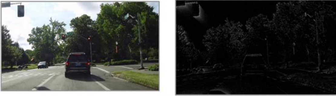
Figure 1.16. The use of retinomorphic sensor on the moving vehicle. It only reflects the image of moving subjects 26 .
