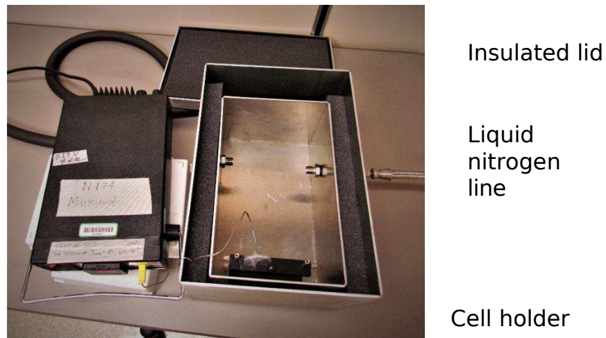
Figure 3. Picture of cooling system for neutron imaging at freezing and below-freezing temperatures.
