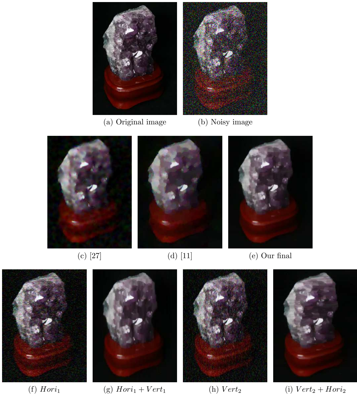
Figure 3.7: Results comparison at image noise level \sigma = 75 . (a) and (b): reference image and noisy image; (c), (d) and (e): denoised result from [27], [11] and our final results. (f),(g),(h) and (i) show the intermediate results during our process – Hori_1 , Hori_1 + Vert_1 , Vert_2 and Vert_2 + Hori_2 . PSNR: [11]=25.8170, [27]=25.4942, ours=29.2042.
