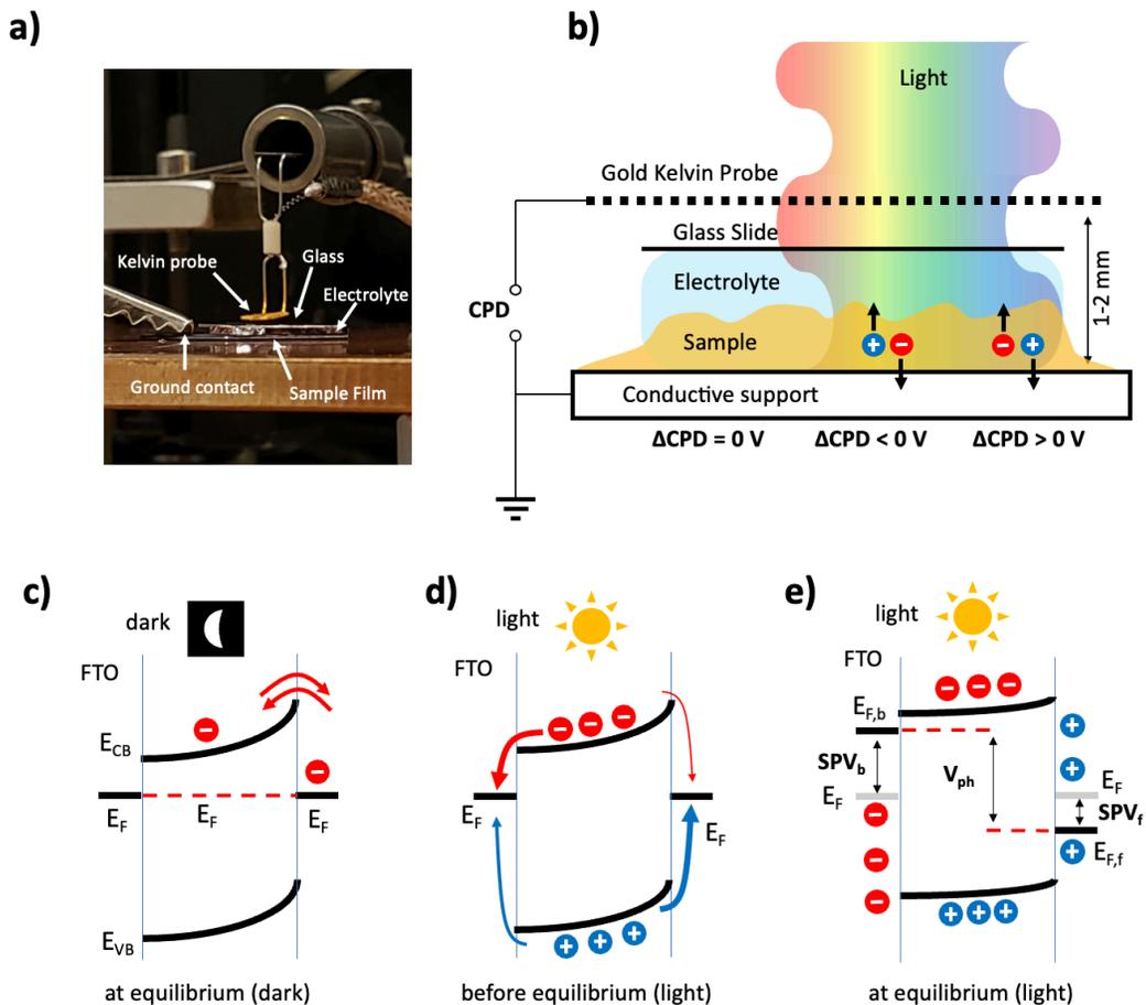
**Figure 2.** a) Vibrating Kelvin Probe Surface Photovoltage (VKP-SPV) Spectroscopy in liquids (Photo.) b) Schematic of the measurement configuration. Sample illumination occurs through the 60% semi-transparent KP, placed 1-2 mm above the sample, and through the electrolyte, enclosed by a microscopy glass cover slide. A water-saturated gas environment serves to prevent drying out of the electrolyte. The Contact Potential Difference (CPD) change under
