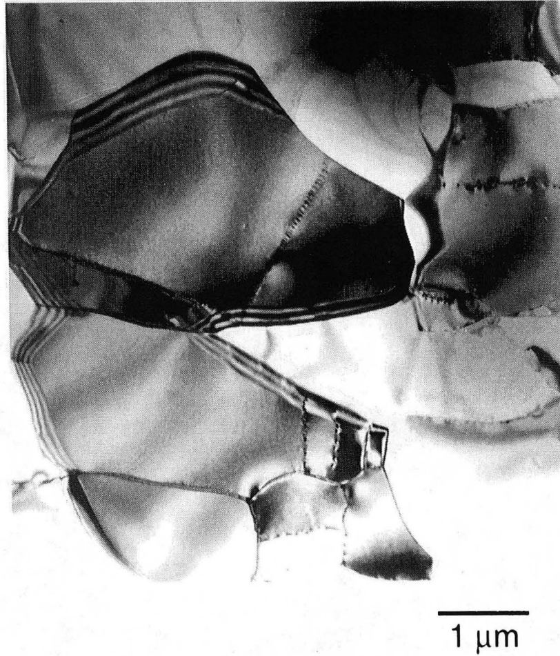
Figure 26: TEM micrograph of the recovered microstructure prior to deformation. Note the existence of some dislocation substructure within the subgrain interior. Zone axis is near [0\bar{1}1] . (XBB 9408-4998)
