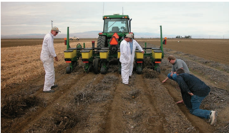
In the 4-year study, researchers successfully established and harvested a cotton-tomato rotation using conservation tillage, with some equipment modifications. Above, a no-till cotton planter (into tomato residue) is evaluated and adjusted.
