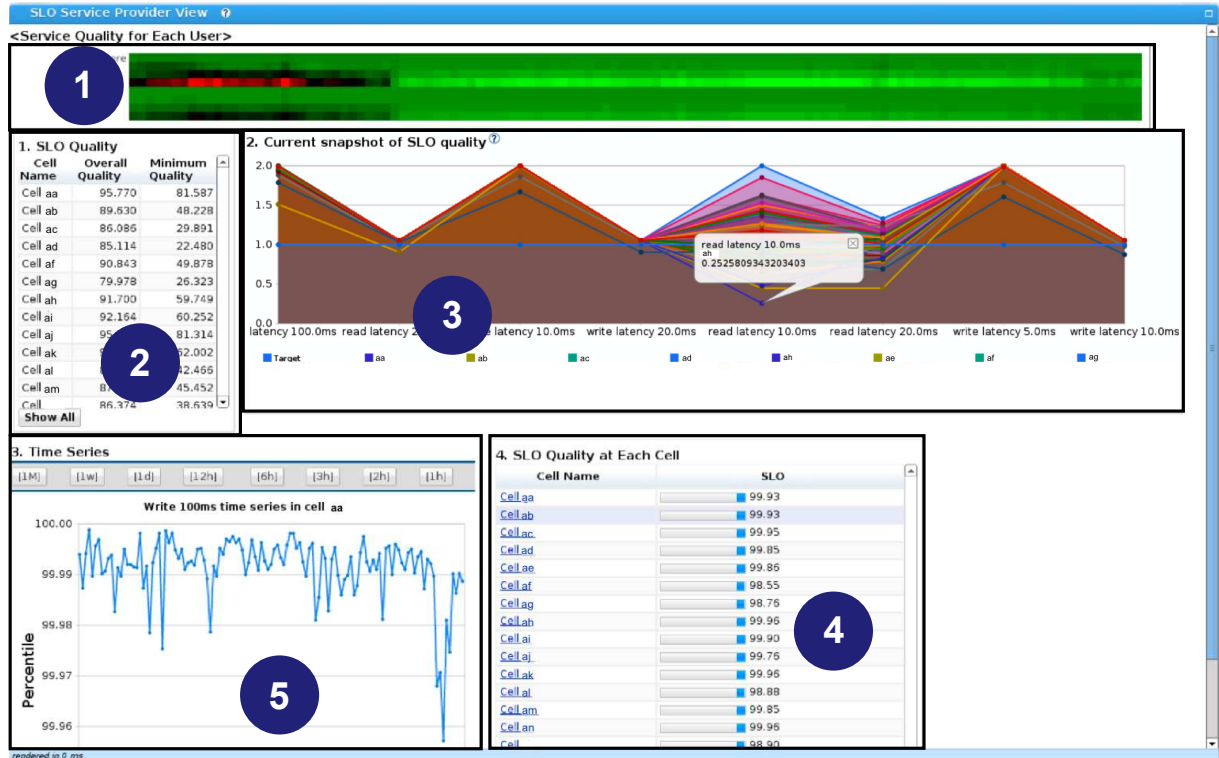
Figure 1: Screenshot of the SLO visualization system. This screenshot shows where each view is placed. The topmost panel (Component 1) is a heat map showing overall SLO quality as a time series. Selecting each row updates the four panels (Component 2–5) below for the selected user. The SLO Quality table (Component 2) shows numerical values for both overall or minimum SLO quality values. The parallel coordinate (Component 3) shows SLO quality values for all SLO line items. The heat map and the parallel coordinate are designed so that they can be used two ways: displaying SLO quality values and providing a way for drill down. The bottommost two panels (Component 4 and 5) display the details as a result of visual exploration. Figure 4 shows the detail about how events update other views. Note that we erased some of our private information from the screenshot, e.g., service names, data center names, and the number of data centers.
