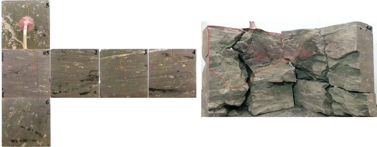
Figure 31. Faces of sample 5 after slick-water fracturing (left) and fracture morphology after gas breakdown. Yellow dashed lines denote the reopened preexisting fractures (left), green dashed lines indicate the epoxy stained area, red curves circle the revealed slick-water fracture plane.
