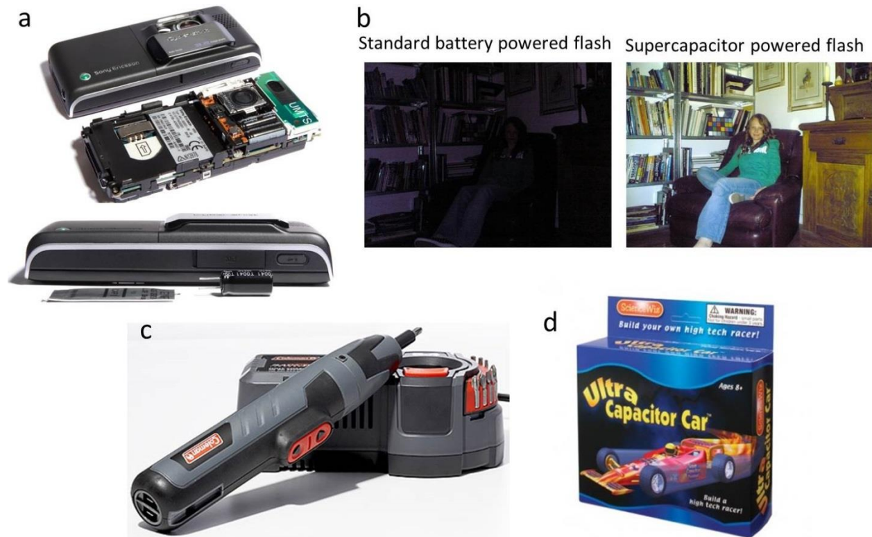
Figure 2.8: Applications of supercapacitors in consumer electronics. (a,b) Camera flash, pictures adapted from (21). (c) Cordless screwdriver, picture adapted from reference (22). (d) Toys, picture adapted from reference (23).
