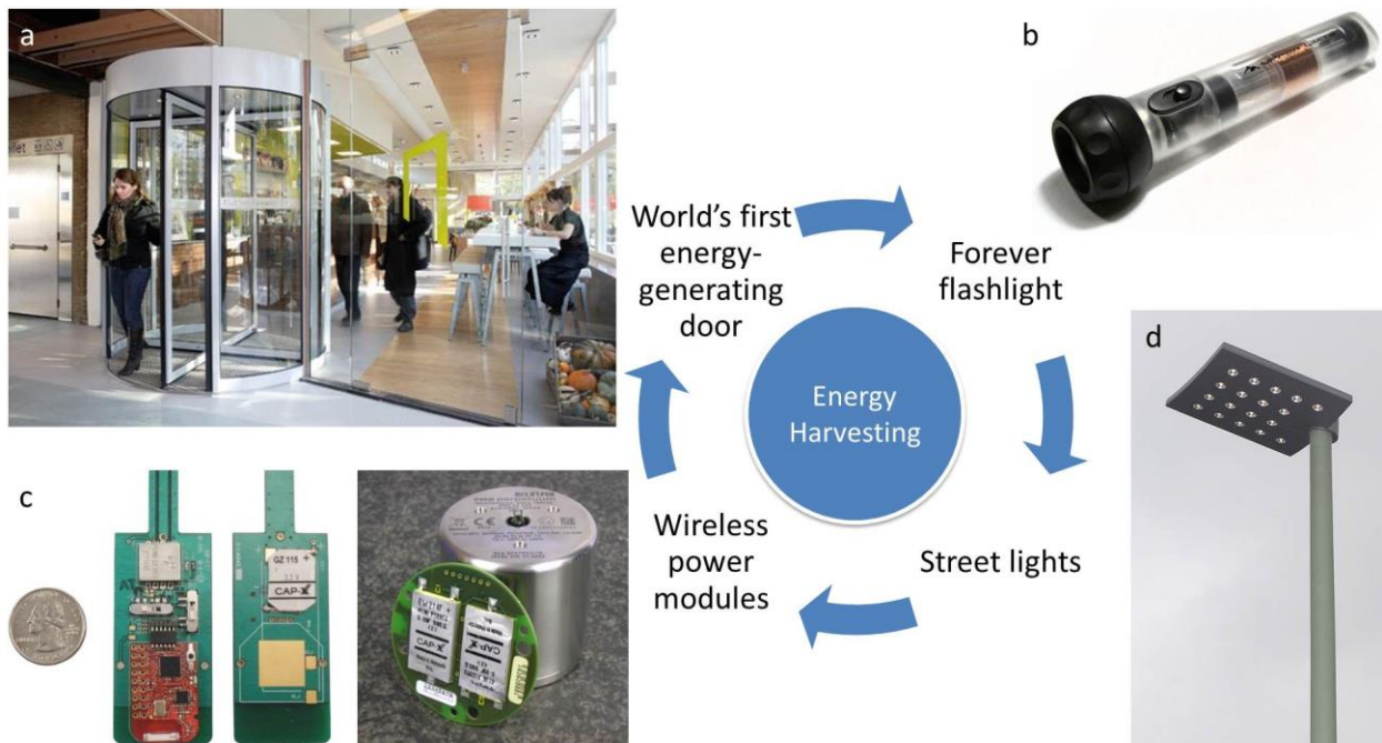
Figure 2.9: Typical applications of supercapacitors for energy harvesting: (a) World's first energy-generating revolving door, Netherlands, adapted from reference (25). (b) A mechanically powered flashlight, adapted from reference (27). (c) Wireless power modules, adapted from (28). (d) A stand-alone power source for a street light, adapted from reference (29).
