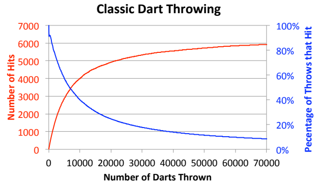
Figure 13: The capability of classic dart-throwing to insert a new point deteriorates as the number of prior darts increases. At 70,000 darts thrown, 90% are rejected. 80% of the accepted darts were thrown during the first 20,000 throws.
