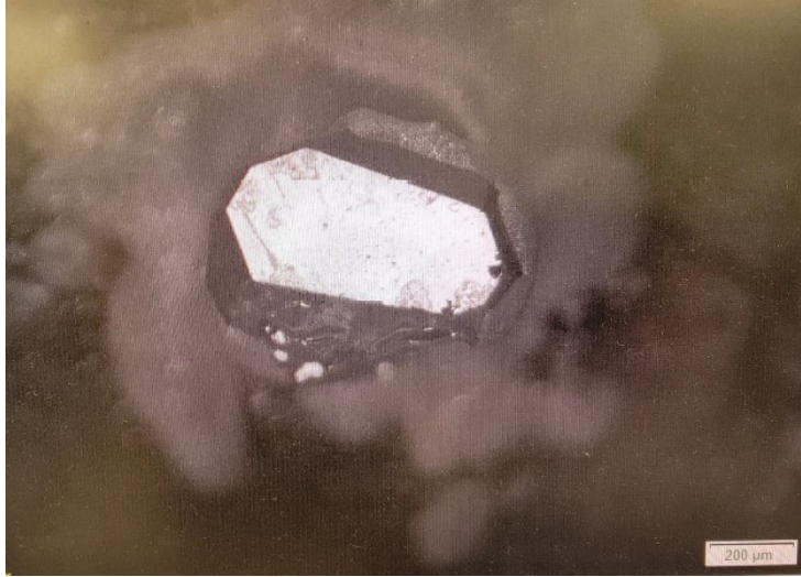
Figure 5.4: The sample of FeGe that was measured by REXS.
