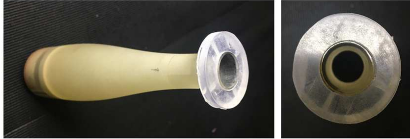
Figure 4.18: Image of the convergent-divergent nozzle with annular end plate.
