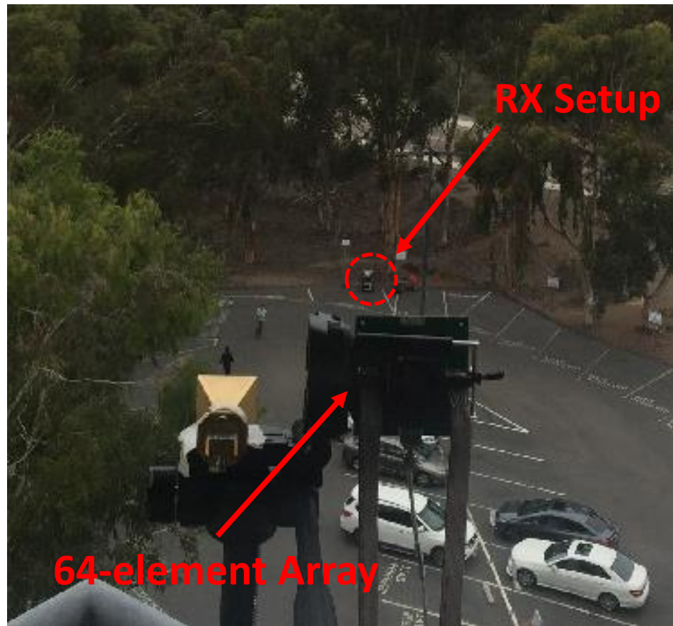
Figure 4.10: Photo of the measurement setup for 90-100 m link.
