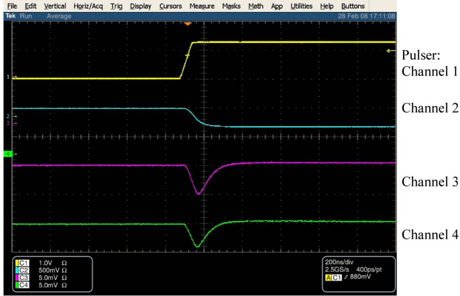
Figure 9: Scope traces of sample signal crosstalk.
