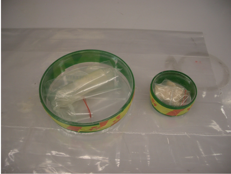
Figure 34: The parylene powder sample (right) and the polypropylene vial in which it was irradiated, bagged, double-contained, labeled, and ready for counting.
