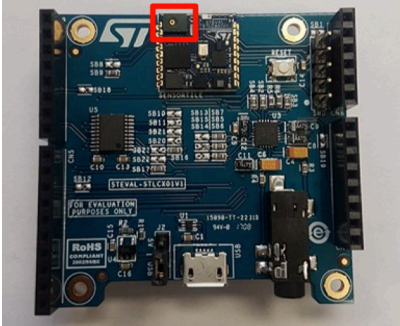
Figure 3.4: Correct mounting of SensorTile on extended crable board
