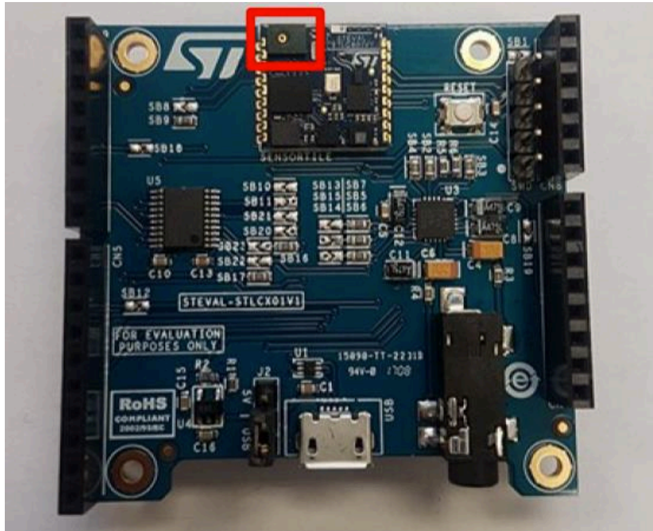
Figure 32: Ensure the orientation of the SensorTile on the larger evaluation board matches this figure. There should be a green protrusion with a little metallic hole right next to the ST logo.
