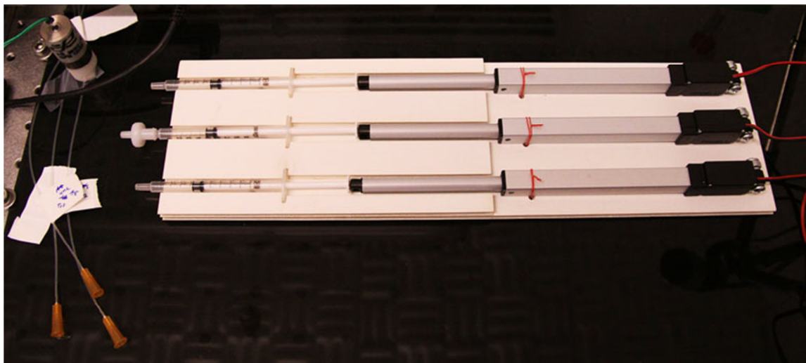
Figure 5.4.1 Low-Cost Syringe Pump Overview
