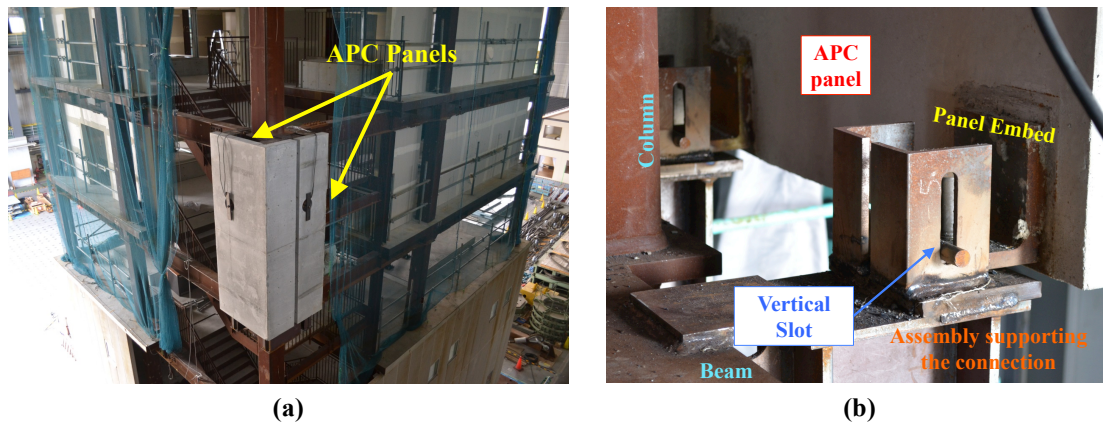
Figure 1.30. E-Defense test on corner APC panels: (a) photograph showing the two panels and (b) photograph of the lower bearing sliding connection (Courtesy of Hutchinson et al. 2014)
