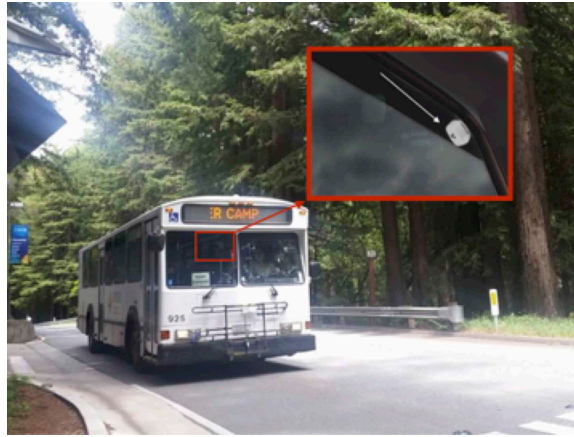
1 2 3 FIGURE 7 A UC Santa Cruz campus bus vehicle that was equipped with a Kontakt.io BLE 4 beacon.
