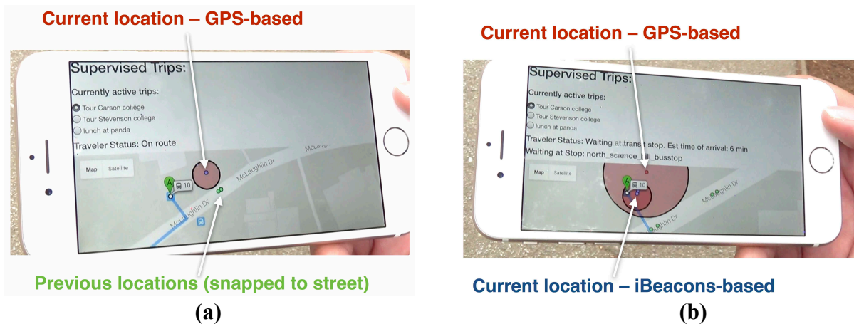
FIGURE 5 Views generated by the web application in two different moments while the traveler was approaching the bus stop marked as ‘A’ in the map. The circles represent the confidence radius for localization provided by GPS or beacons.
