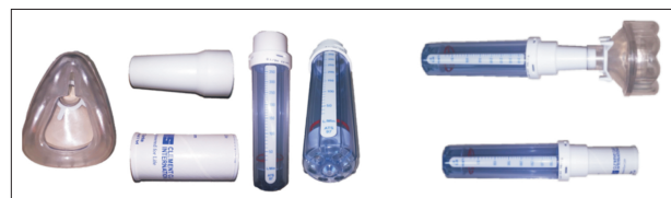
Figure 2. In-Check medical device. The left image shows the disassembled parts of the In-Check medical device. The right image shows the assembled In-Check medical device for peak nasal inspiratory flow (with nasal mask) and peak oral inspiratory flow measurements (with disposable oral mouthpiece).
