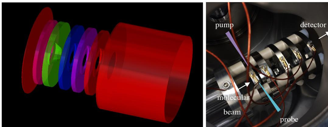
Figure 2-1. Velocity map imaging electrodes incorporating conical extractor design
