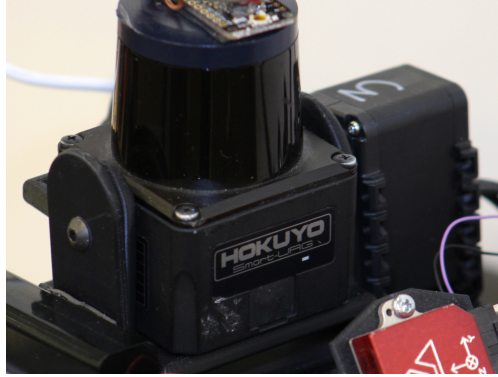
Figure 4: Our mapping solution consisting of a 2D lidar mounted on a nodding gimbal.
