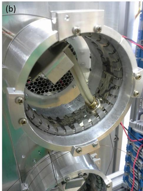
Figure A.1. Schematic and photo of miniature gas chromatographs. Clamps on the edges of the rim of the hub hold the chromatography column in place at each end. An aluminium sheet is wrapped around the outside of the hub over the column to further ensure even heating of the column itself.
