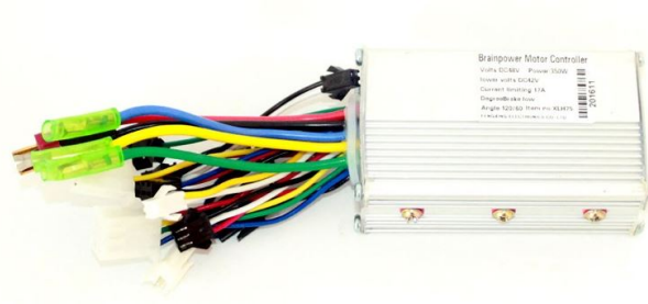
Figure 4.2: Electronic Speed Controller
