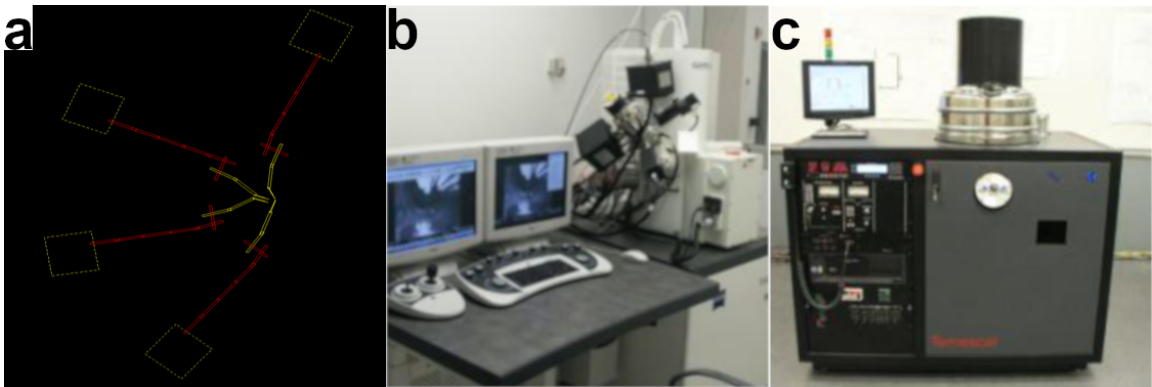
Figure 3.12: Essential procedures and equipment for producing graphene-MoTe 2 -graphene optoelectronic devices through EBL. (a) DesignCAD 2000 and NPGS design for electrical contacts on a heterostructure device. (b) Leo XB1540 focused ion beam milling system, used for pattern writing. (c) Temescal BJD 1800 e-beam evaporator, used for metal deposition.
