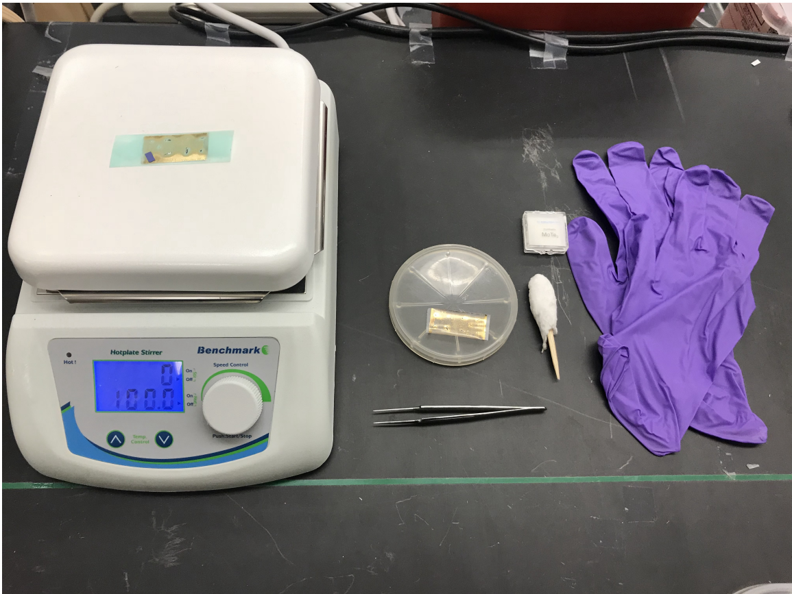
Figure 3.8: Equipment and materials used in the gold assisted method of exfoliating atomically thin materials.
