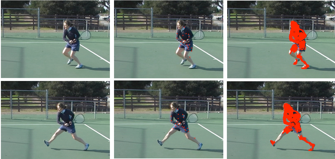
Figure 6.9: (Top) Frame 490 of the tennis sequence with (left) actual image, (middle) KLT points and (right) LDOF points. (Bottom) Frame 495 of the sequence with (left) actual image, (middle) KLT points and (right) LDOF points. Only points on the player are marked. KLT tracker points are marked larger for easy visual detection. Figure best viewed in color.
