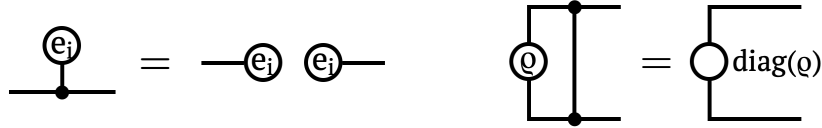
Figure 4.1: Left: using a third-order copy tensor contracting with a basis state vector results in an outer product of the basis vector, which can be thought of as conditioning on the same basis state upon contraction with two nodes. Right: Obtaining the diagonals of a density matrix, or a matrix in general, can be done by contracting the matrix with two third-order copy tensors and contracting one bond of each of the copy tensors together.
