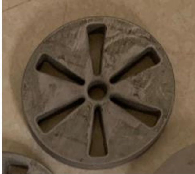
Figure 14: 81% blockage ratio turbulence intensity generator
