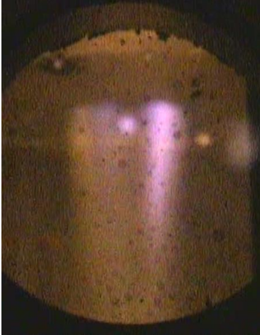
Figure 10: 50% H 2 -50% CO jet flame retracting (i.e. flashback)
