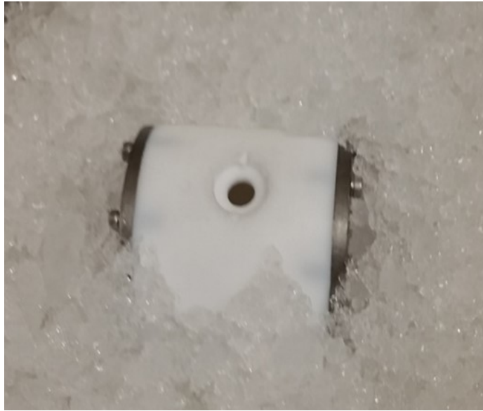
Figure 3.9: A photograph demonstrating the "vertical method" of etching in which a Nb end-cap is affixed to each end of a Teflon tube in the same manner as described in Fig. 3.8. A hole is drilled into the side of this Teflon tube and it is then laid onto its side so that the BCP solution can be poured into the hole. This method is an attempt to mitigate the problem of material settlement described in the "cup method" BCP summary.
