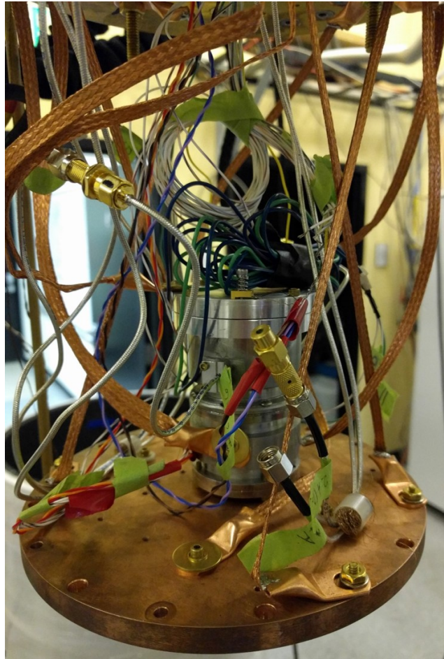
Figure 4.1: A photograph of the sample container space where we place our cavities for cryogenic testing. The SMAs feed through the plates separating temperature stages of the DR and connect to the cavity input/output couplers. Copper braids are attached to the cavity body and act as thermal anchors to ensure heat exchange takes place as the system is under vacuum during testing.
