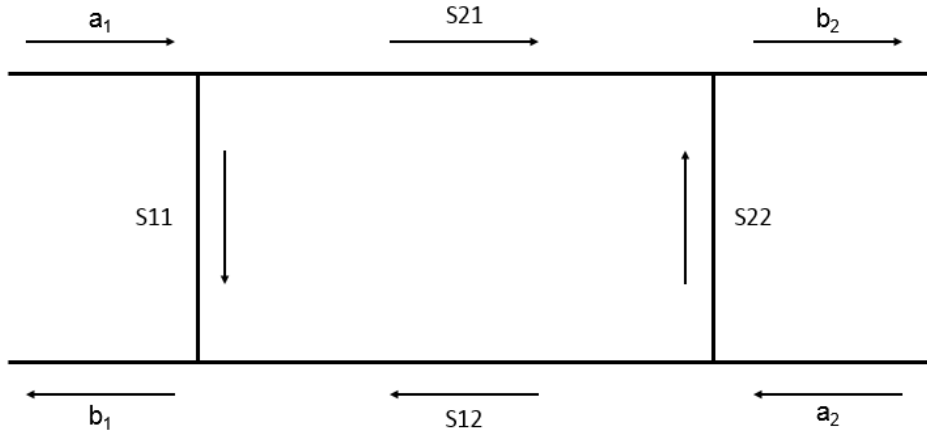
Figure 4.2: A diagram of outgoing ( a_n ) and incoming ( b_n ) power waves in a two-port microwave circuit. The S-parameters follow the labeling convention S_{n_b n_a} where n represents the port number, a is a wave leaving the port, and b is a wave going into the port. We are only interested in reflection ( S_{11} ) and transmission ( S_{21} ) measurements. That is, we use the output signal from port 1 to measure the cavity reflection spectrum at port 1 or the cavity transmission spectrum at port 2.
