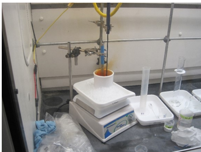
Figure 3.7: A photograph demonstrating the "dunking method" of etching in which the BCP solution is contained within a Teflon beaker which is in turn placed in an ice bath in an attempt to control the temperature of the reaction. As evidenced by the orange smoke, this method is prone to thermal run-away even when taking necessary precautions due to the large surface area that is exposed to the BCP solution.
