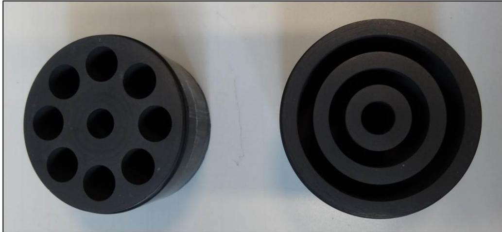
**Figure 4.7** – Photographs of the experimentally-implemented Holes (left) and Rings (right) setups.
