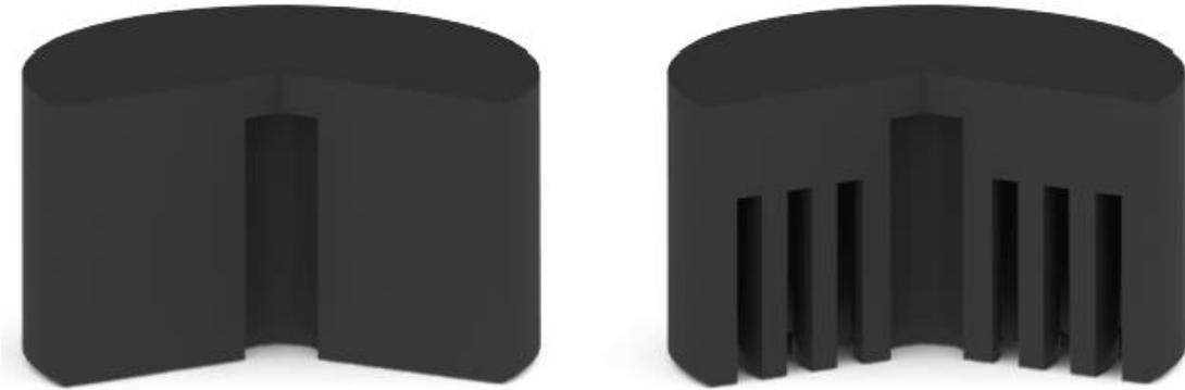
**Figure 4.19** – Comparison between the Full and optimized 3 Rings punches.
