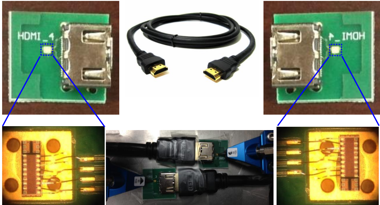
Fig. 3.6 Complete channel with package, transmission line on PCB, and HDMI Connect/Cable modeling
