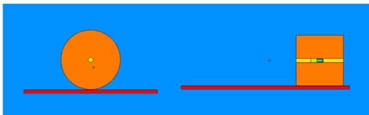
Figure 6-9 From left: axial view of the 16 cm CTDI phantom geometry built in MCNPX and sagittal view with visible ion chamber in the center. Red bar represents the table built as a 1 cm thick carbon board.
