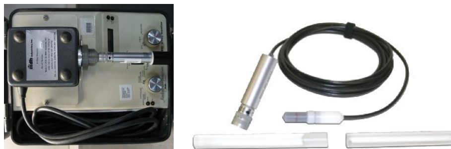
Figure 6-5 MDH 1015 and 0.6cc ionization chamber used for the measurements (courtesy of RadCal).
