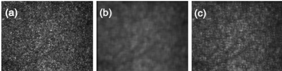
Figure 3.3: Examples of: (a) ground truth image; (b) blurry image; (c) corrected image. The NMSE were: (b) 0.042 (c) 0.020, and the SSIM: (b) 0.28 (c) 0.58.
