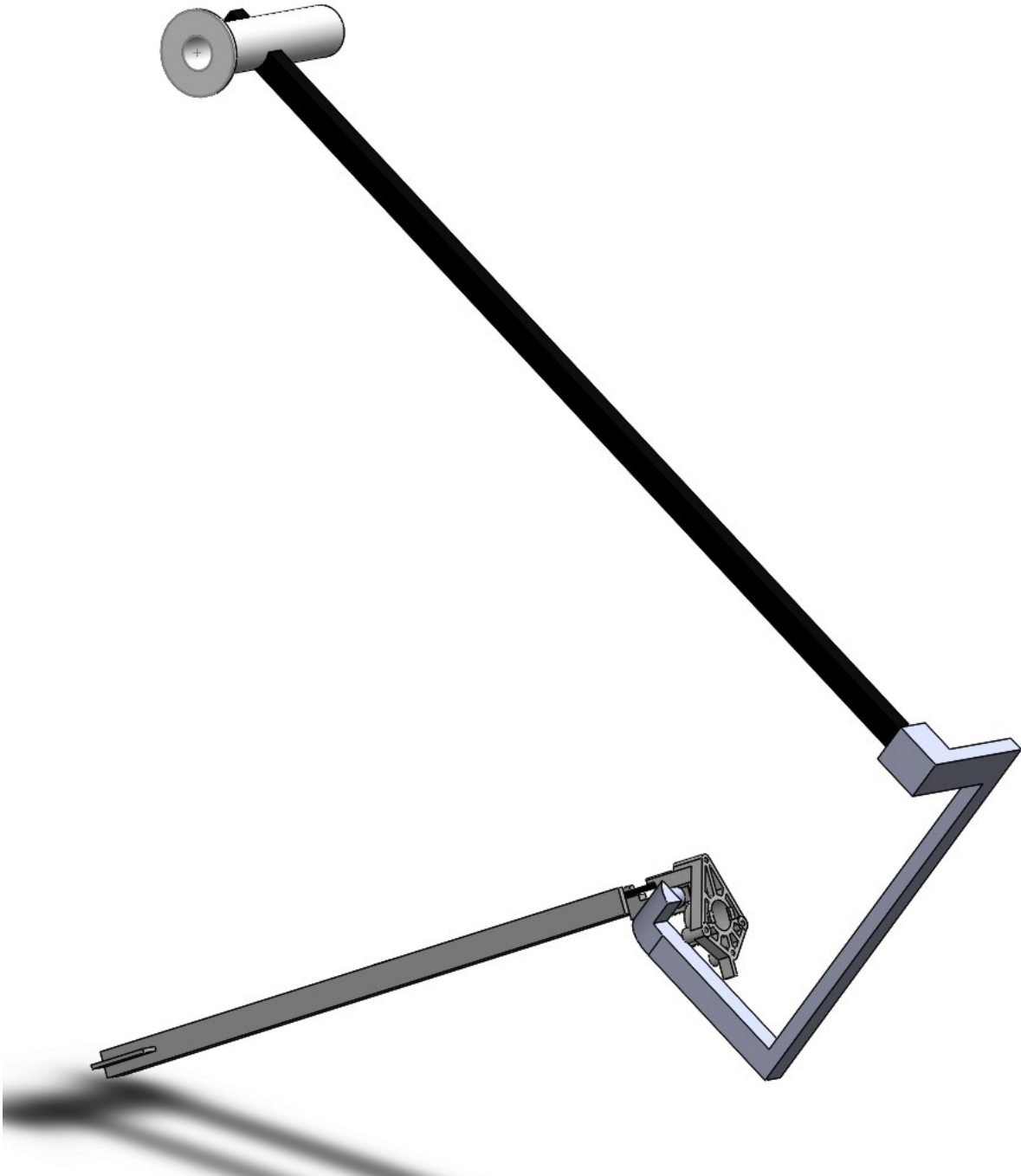
Figure 4.18: Simplified schematic of the setup from the hall sensor mount to the body of flapping setup
