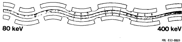
Fig. 5 Calculated ion trajectories through a TFF accelerator. Arrows show the direction of the electric force.
