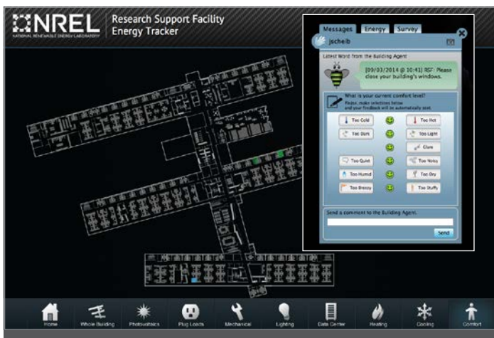
Figure 5-1. NREL’s formal occupant-operator communication system. Left: Webpage for operator to view comfort reports and feedback from the occupants. This information can be used to make decisions about system change requests or operations issues. Inset: Software application for occupants to report comfort information to the operator.
