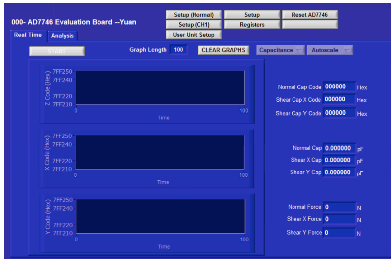
Figure 36 Screenshot for LabVIEW program user interface for testing AD7746
