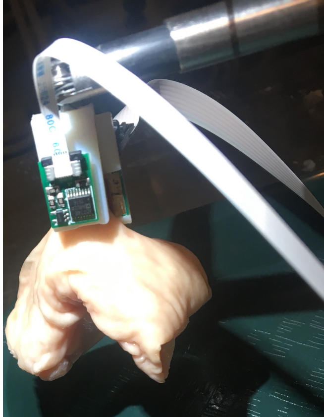
Figure 76 Ex-vivo porcine large intestine handled using da Vinci IS1200 Cadere forceps
