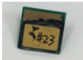
Figure 34 The sensor is contacted with the sensor board grounding area with PS:PTT, but not conducting
