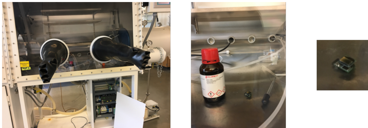
Figure 35 (left) The glove box which we applied the Poly (3,4-ethylenedioxythiophene)-poly(styrenesulfonate) (middle) the conductive polymer, the sensor, and the glass tube that used to apply the conductive polymer
