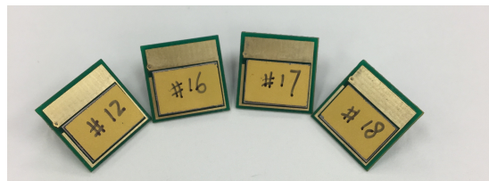
Figure 33 The grounded sensor board and gold deposited assembled sensor
