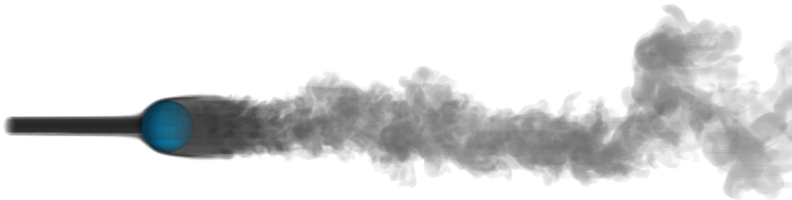
Figure 3.22: Visualization of a passively advected smoke marker in a flow past a sphere for a Reynolds number Re = 5,000 .
