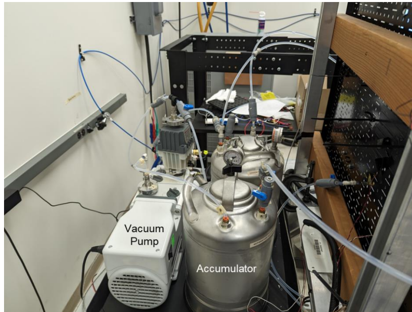
Fig. 10. Experimental setup of Accumulator and Vacuum pump.
