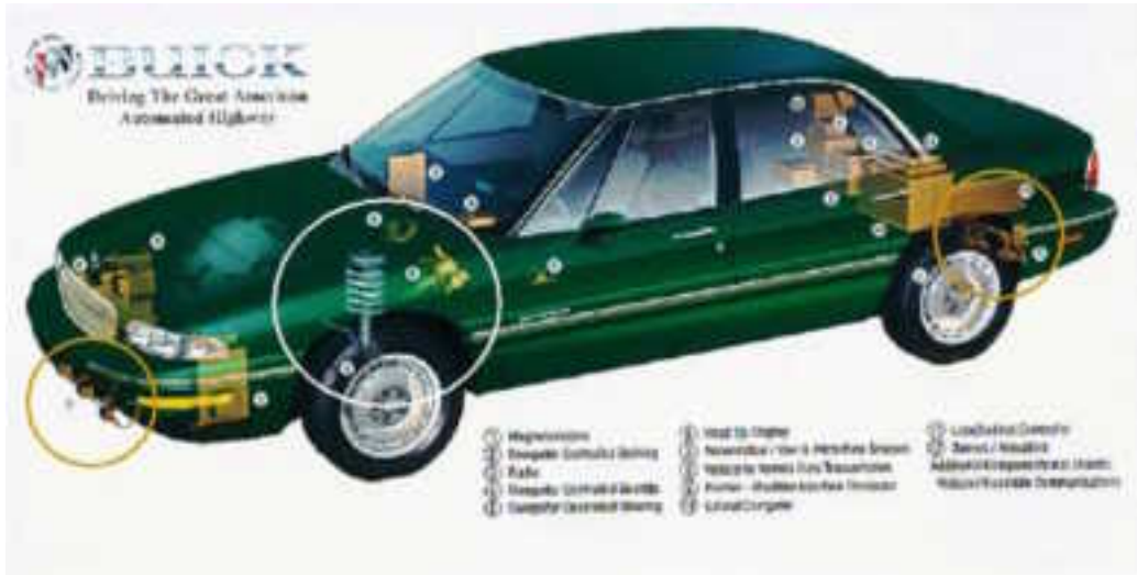
Figure 2: Hardware configuration on passenger vehicles. Smaller circles encircle magnetometer locations. Larger circle encircles the "inner-loop"
