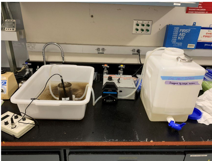
Figure 4. Photo of the process used to fill peat cores. A Geotech pump (middle) delivered the incubation water from the reservoir (right) to the bottom of the core (left). Water was allowed to flow up and out of the core. A conductivity electrode confirmed when the conductivity within the core was equal to the incubation water
