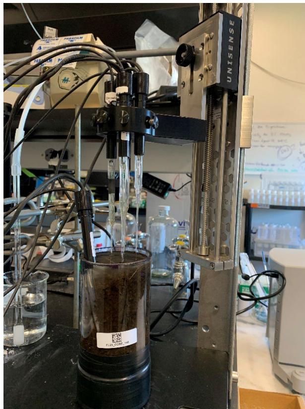
Figure 6. Photo of peat core being microprofiled with microelectrodes. Electrodes profile vertically 6 cm downwards from the water surface at a measurement interval of 250 \mu\text{m} .
