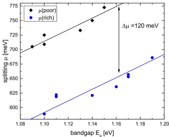
FIG. 3. QFLs of Cu-poor (black diamonds) and Cu-rich (blue circles)  $\text{Cu}(\text{In,Ga})\text{Se}_2$  absorber layers plotted against their electrical bandgap measured under illumination equivalent to two suns. The solid lines represent linear fits with a fixed slope of 1.
