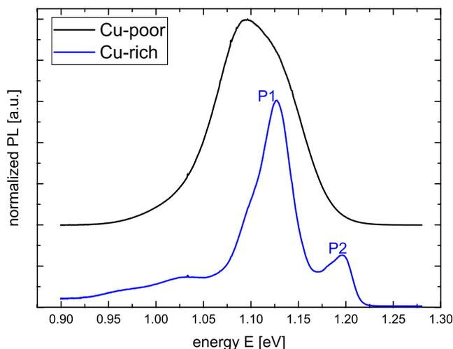
FIG. 1. Measured photoluminescence spectra of a Cu-poor (top, shifted upwards for better visibility) and a Cu-rich (bottom) Cu(In,Ga)Se<sub>2</sub> absorber at 10 K.
