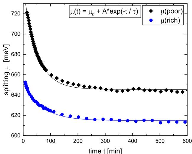
FIG. 2. QFLs  $\mu$  of a Cu-poor (black diamonds) and a Cu-rich (blue circles) Cu(In,Ga)Se<sub>2</sub> absorber after etching as a function of time. Solid lines are exponential fits with the displayed equation according to the work of Regesch *et al.*<sup>9</sup>
