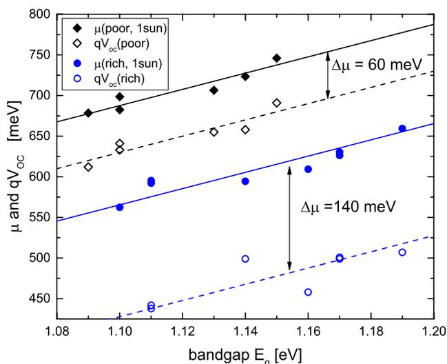
FIG. 5. QFLs of Cu-poor (closed diamonds) and Cu-rich (closed circles) Cu(In,Ga)Se<sub>2</sub> absorber layers as well as the corresponding  $V_{oc}$  (open symbols) for 1 sun illumination.
