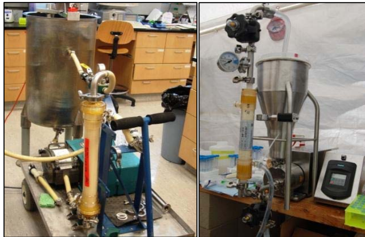
Figure 5. Laboratory setups of large (left) and small (right) hollow fiber ultrafiltration systems
