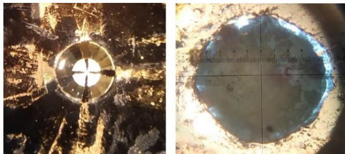
Figure 13. On the left: Diamond with gold sputtered contacts (no sample). On the right: IBN sample within a gasket hole at 5 GPa. The PVC layer is seen in the transparent light blue areas between the inner gasket hole and sample.
