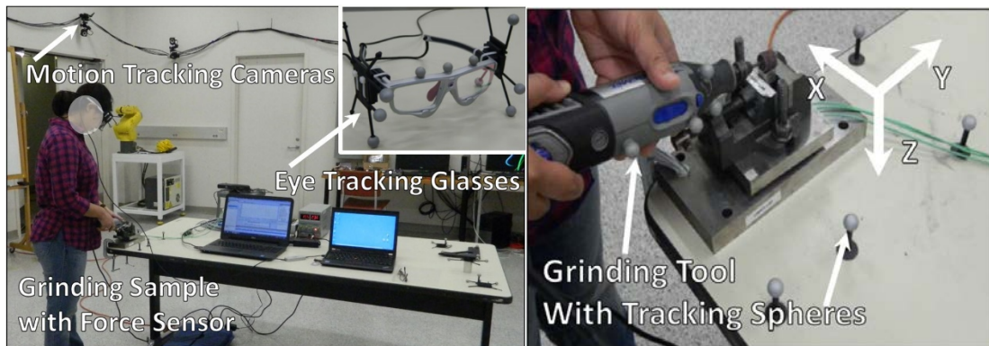
Fig. 4. Experimental Setup consists of eye tracking glasses, kinematic sensors, camera, and piezoelectric force sensor, reprinted from [4].
