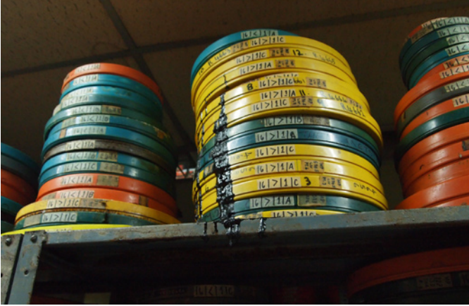
Fig. 3. Black ooze can be seen dripping from film canisters stored at the PIA Film Vault.
