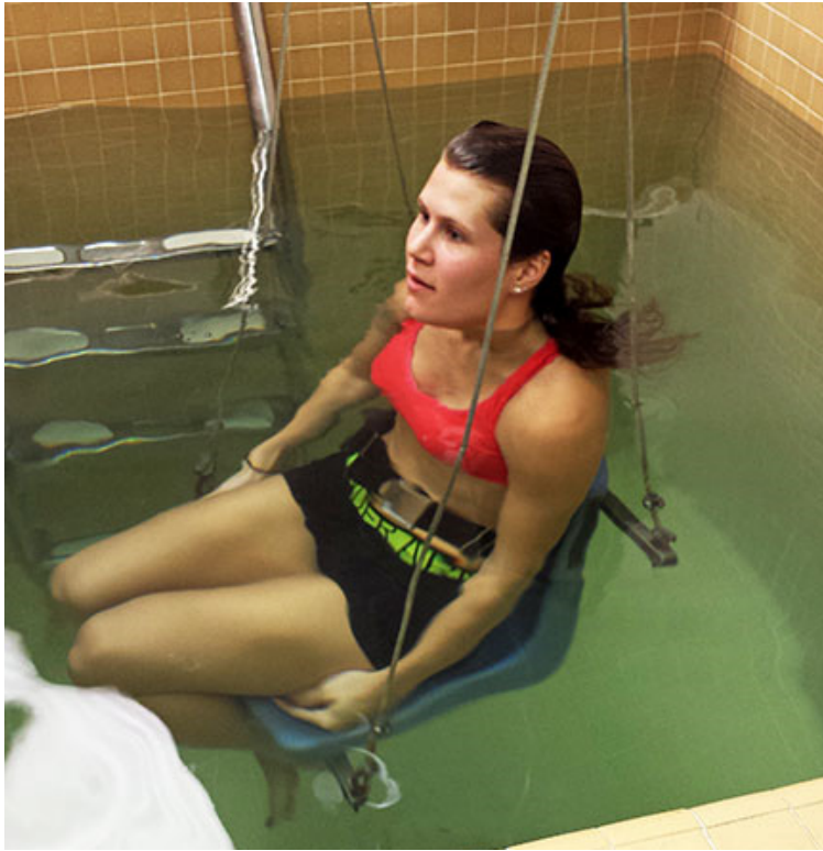
Figure 3-1: Example of an underwater weighing apparatus. The subject rests on a seat connected to a force meter. The seat is lowered into the water until the subject is completely submerged, and her underwater weight is then measured. Image source: https://education.uky.edu/khp/laboratories/exercise-physiology-lab/
