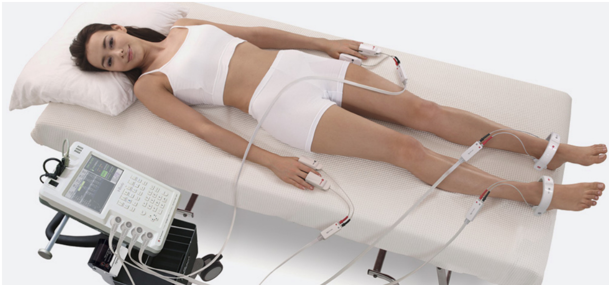
Figure 3-3: A clinical multifrequency segmental bioelectrical impedance analysis device with touch electrodes connected to the subject's fingers and ankles. InBody S10 (InBody Co. Ltd., Seoul, South Korea). Image source: http://www.inbody.com/global/product/inbodys10.aspx
