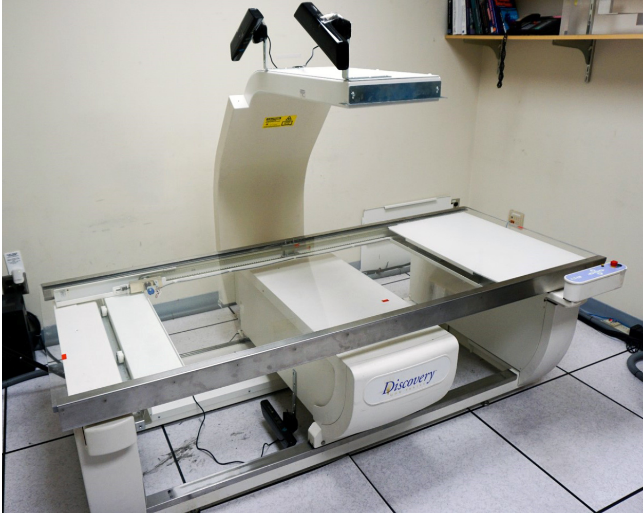
Figure 6-8: Prototype Ultra DXA system with integrated transparent acrylic tabletop and 3D depth cameras.
